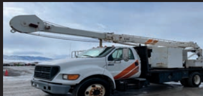
Smeal 10T Pump Hoist, p/b Cat 3126 6 Cylinder, 246 HP, Mntd on 2001 F-750 Trk, 36' Tele. Mast...$87,500
