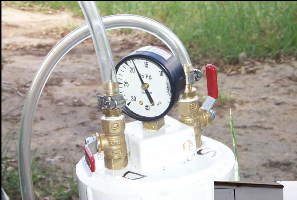
Sampling Headspace of North Water Well
