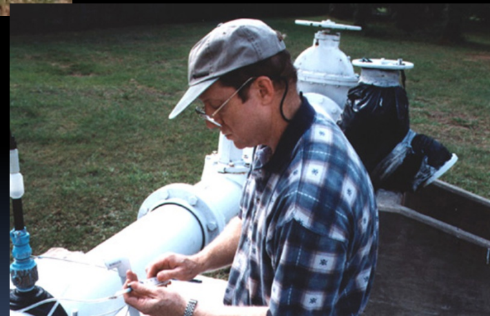
Sampling MUD Well-Casing Headspace and Ground Water
