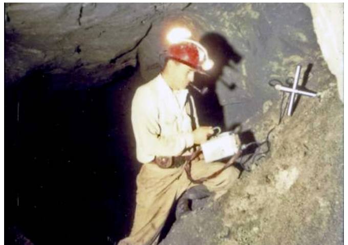
Figure 4. Grade control engineer checking the grade of blasted ore with a T-probe (grade control instrument) at the Dysart No. 1 mine, Ambrosia Lake subdistrict, McKinley County. Photo by K.G. Hatfield in the late 1950s.
