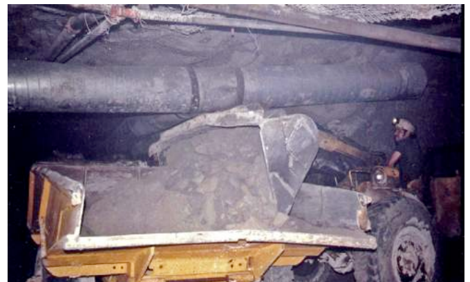
Figure 6. Dump truck being loaded with ore at the Homestake-Sapin Partners Section 25 mine, Ambrosia Lake subdistrict, McKinley County. Photo by U.S. Atomic Energy Commission geologists in the 1960s.
