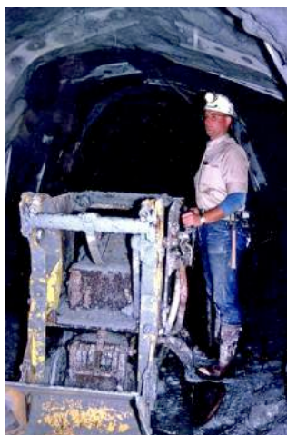
Figure 7. Mine official showing visitors how an overhead mucking machine operates at the Homestake mine, Ambrosia Lake subdistrict, McKinley County. Photo by U.S. Atomic Energy Commission geologists in the 1960s.
