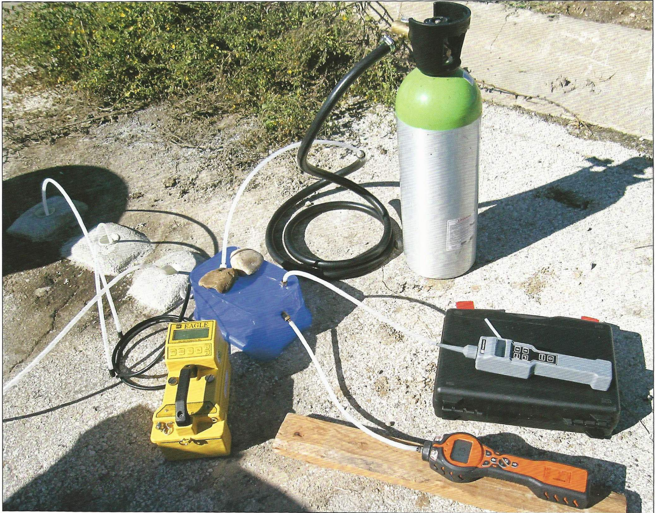
Leak detection testing using helium gas
